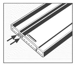
The rear of the toekick has two cutting lines.
